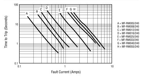
The Time to Trip curves represent typical performance of a device in a simulated application environment.
